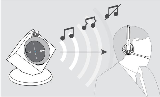
In normal office buildings, the range between headset and base station is up to 55 m.
