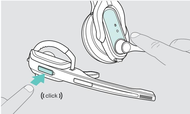
> Press the Link button on the headset to disconnect an existing wireless link between base station and headset. The LEDs on the headset and on the base station go off.
