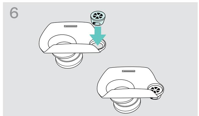
> Re-mount ear hook interface – if required – by pushing it in from the backside of the adapter.
