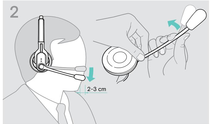
> Bend the microphone boom so that the microphone is about 0.8" (2 cm) from the corner of your mouth.
