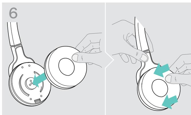
> Reattach the ear pad to the ear cup by pressing firmly around the ear pad.
