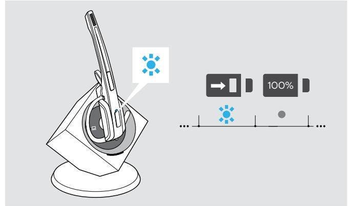
The Headset LED lights up blue and the rechargeable battery is being charged. The Charge status LED on the base station indicates the charge status.
