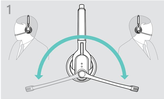
> Rotate the microphone boom.
