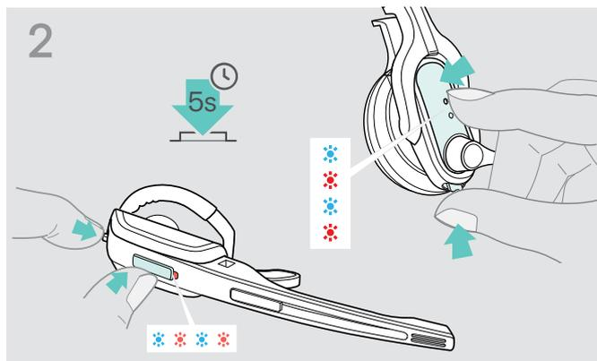
> Simultaneously press and hold the Link button and the Audio button for 5 seconds. The Headset LED alternately flashes blue/red.
