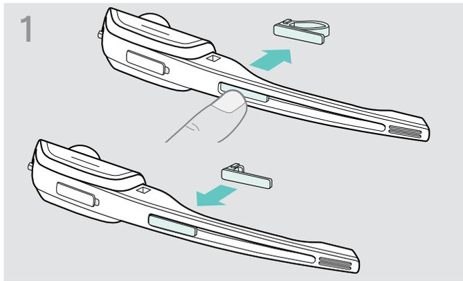
> Replace the name plate with cheek spacer with the basic name plate. This is necessary in order to be able to rotate the headset's microphone boom (see diagram 3).
