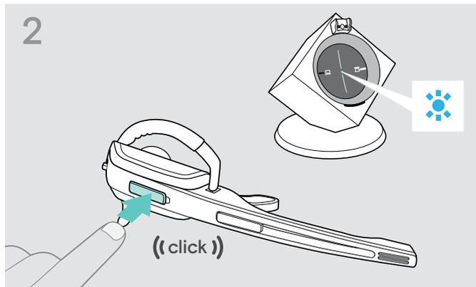
> Press the Link button on the headset. The Link LED lights up blue
