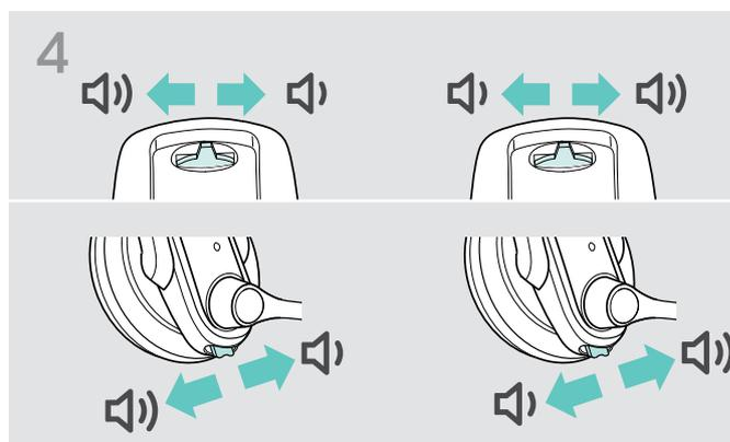
The direction of the volume up/down function of the Audio button is changed. The headset switches to standby mode.
