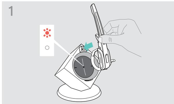
The Link LED on the base station is off (headset is disconnected) or lights up red (no headset paired).
