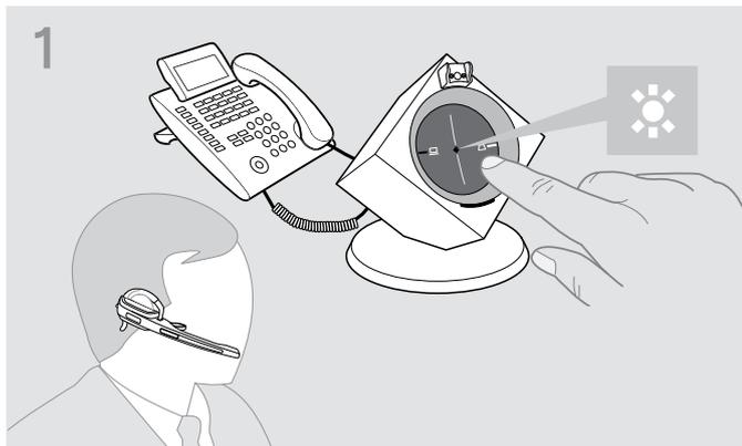
> Put on the headset and press the Phone button on the base station.
