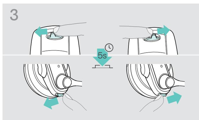
> Push the Audio button in the direction “volume down” until the Headset LED goes off.
