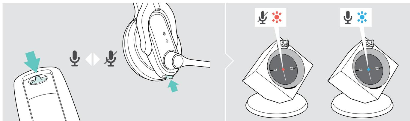
> Press the Audio button. The microphone is muted. While the microphone is muted, the Link LED on the base station flashes red.
