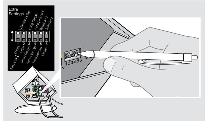
> Use a pointed object (e.g. a ball pen) to set the DIP switches to the desired position.
