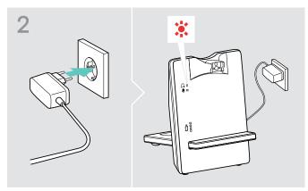
Connect the power supply unit to a wall socket. The Link LED lights up red.
