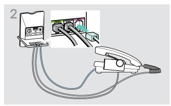
> Connect the handset lifter to the fixed line phone. For more information, refer to the instruction manual of the HSL 10 II handset lifter.
