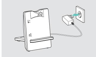
Disconnect the base station from the mains power supply. The base station switches off immediately the based
