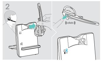
> Take the headset out of the base station and press the Link button to connect the headset with the base station.
