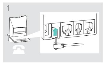
> Connect the plug of the power supply unit to the DC IN socket (marked yellow).
