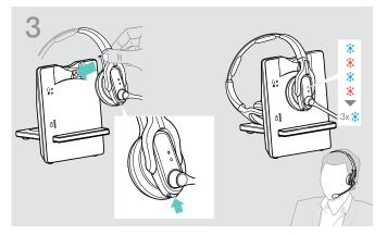
> Press and hold the Audio button while placing the guest headset into the base station of the master headset. The Headset LED alternately flashes blue/red until a link to the base station is established. The Headset LED flashes blue 3 times. The headset system allows you to make a conference call with up to 4 headsets from the D-series.
