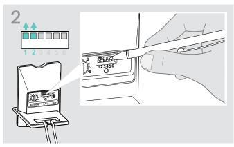
> Use a pointed object (e.g. a ball pen) to set the DIP switches 1 and 2 to the position shown.
