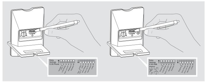
> Use a pointed object (e.g. a ball pen) to set the DIP switches to the desired position.
