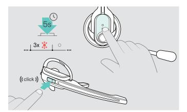
> Press and hold the Link button for 5 seconds to switch off the headset immediately. The Headset LED flashes 3 times red, the headset is switched off completely. The Link LED on the base station lights up red after a short time, the Charge status LED on the base station goes off.
