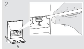
> Use a pointed object (e.g. a ball pen) to set the DIP switch to the position shown in the cable Quick Guide.
