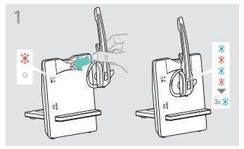
> Place the master headset into the base station. The Headset LED alternately flashes blue/red until a link to the base station is established. The Headset LED flashes blue 3 times.
