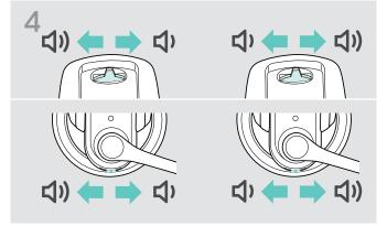
The direction of the volume up/down function of the Audio button is changed. The headset switches to standby mode.
