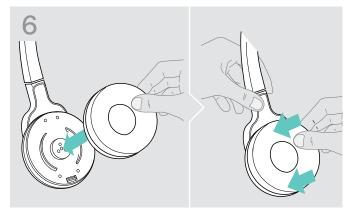
> Reattach the ear pad to the ear cup by pressing firmly around the ear pad.
