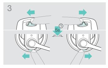
> Push the Audio button in the direction "volume down" until the Headset LED goes off.
