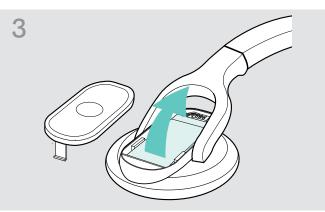
> Remove the rechargeable battery and carefully loosen the connector plug of the rechargeable battery.
