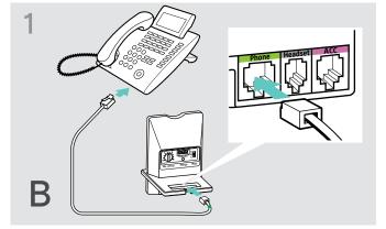
Connect the telephone cable to the headset socket on the telephone and to the Phone socket (marked green) on the base station.
