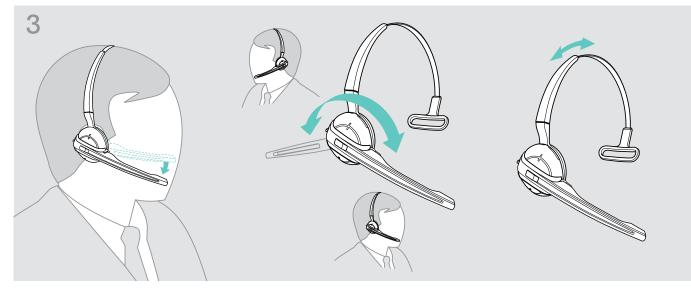
> Rotate the microphone boom and adjust the headset so that the ear pad rests comfortably on your right or left ear.
