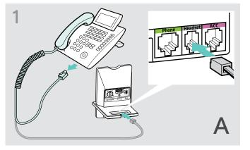
> Disconnect the handset cable from the telephone and connect it to the Handset socket (marked gray) on the base station.
