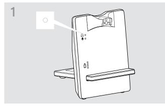
Make sure that the headset is in standby mode (the Link LED on the base station is off). If necessary, press the Link button on the headset.
