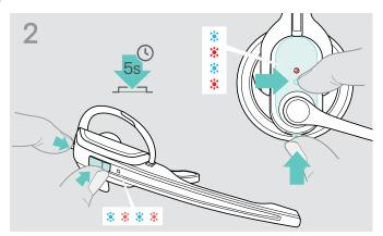
Simultaneously press and hold the Link button and the Audio button for 5 seconds.
