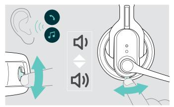
Move the Audio button as shown in the diagram, to adjust the volume.
