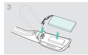
Insert the connector plug of the new rechargeable battery into the connection socket. Observe correct orientation of the connector plug.
