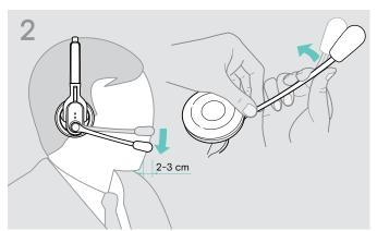
> Bend the microphone boom so that the microphone is about 0.8" (2 cm) from the corner of your mouth.
