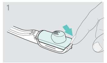
Remove the earhook or the headband (see page 13) and open the battery compartment.
