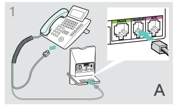
> Disconnect the handset cable from the telephone and connect it to the Handset socket (marked gray) on the base station.
