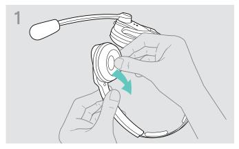
> Carefully remove the ear pad from the ear cup where the battery compartment is located.
