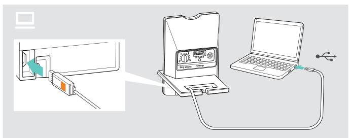
> Connect the USB cable to the PC socket (marked orange) on the base station and to a USB socket of your computer. The operating system detects the USB audio device and installs the necessary drivers.
