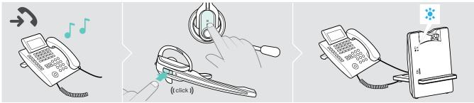
> Press the Link button on the headset to accept the call. The handset lifter/electronic hook switch lifts the handset.
