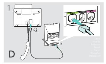
> Connect the base station to the fixed line phone as shown in the cable Quick Guide.
