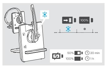
The Headset LED lights up blue and the rechargeable battery is being charged. The Charge status LED on the base station indicates the charge status.
