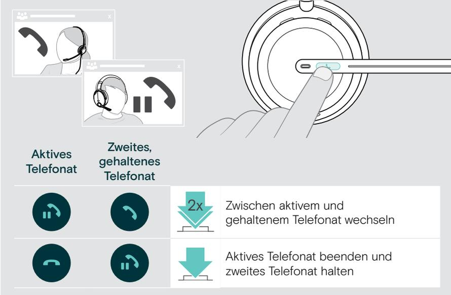
The diagram illustrates the process of switching between active and held calls using a headset. At the top left, two call windows are shown: one with an active call icon and another with a call icon and a pause symbol. To the right, a hand is shown pressing a button on a headset. Below this, a table explains the call management actions:
