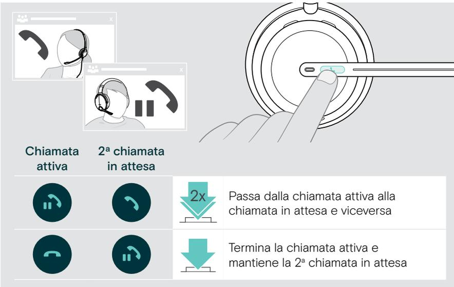
The diagram illustrates call management on a headset. It features two call windows: one with an active call icon and another with a call on hold icon. A hand is shown interacting with a touch-sensitive button on the headset. Below this, a table defines the actions for each call state.
