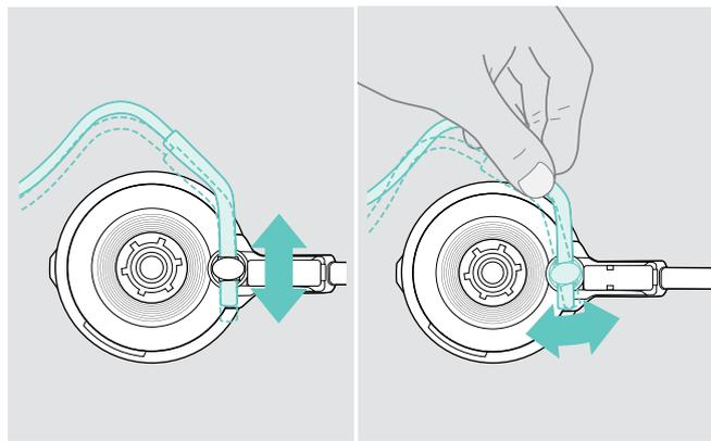
▷ Adjust the neckband's height and angle.
