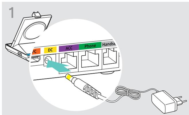
▷ Connect the plug of the power supply unit to the DC socket (marked yellow).
