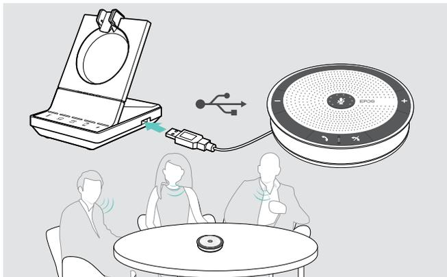
To use an **external speaker with microphone** such as the EPOS speakerphone SP 20:
