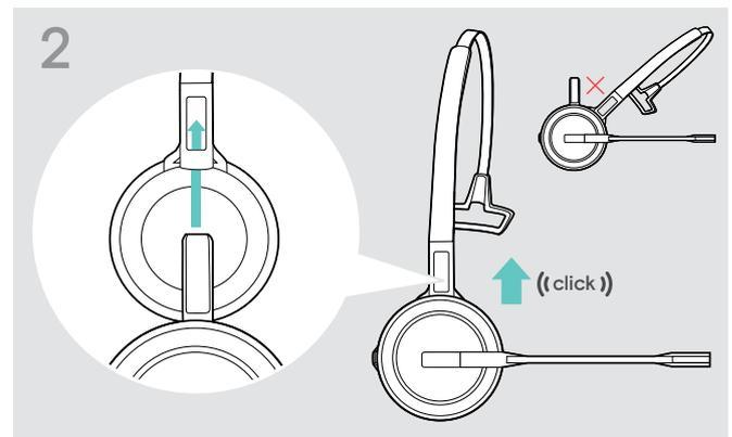
▷ Slide the charging pin into the holder of the headband.
