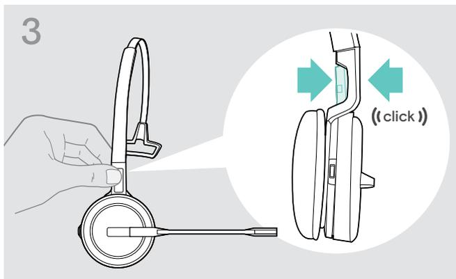
▷ Snap the charging pin into the headband.
