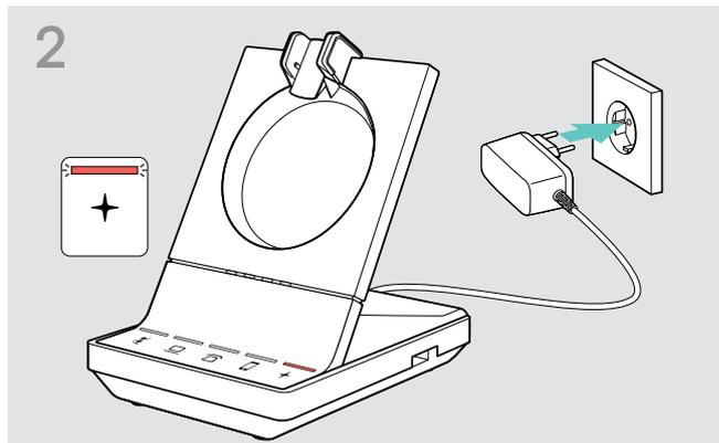
▷ Connect the power supply unit to a wall socket. The + LED lights up red. See page 13 for supported features with and without power supply connection.
