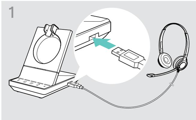
▶ Connect the headset to the **USB** socket on the base station.
